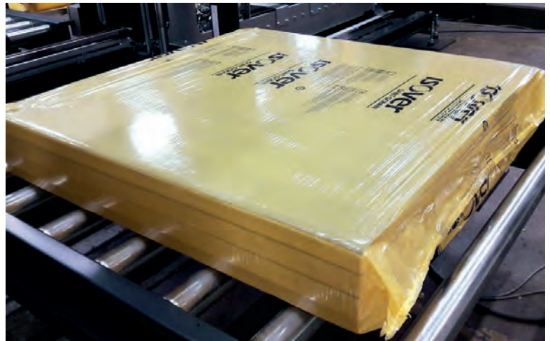
The Isover mineral wool packed and sealed using the RoRo StretchPack® machine.
