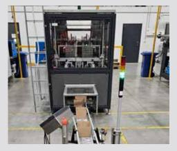
• To achieve Inex's goal, SEE specified its I-Pack® Void Reduction System. The automated solution has been specifically designed for high-volume E-Commerce fulfilment, where packaging efficiency, speed and protection are crucial
